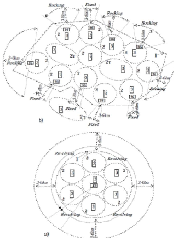
**Figure 5** An outline of a version of wide-ranging anti-hail protection network with far-detection systems 1 – a protected area, 2 – a protected site, 2T – a trapping area, 3 – an anti-hail protection system, 36 – a far-range detector-alerter
