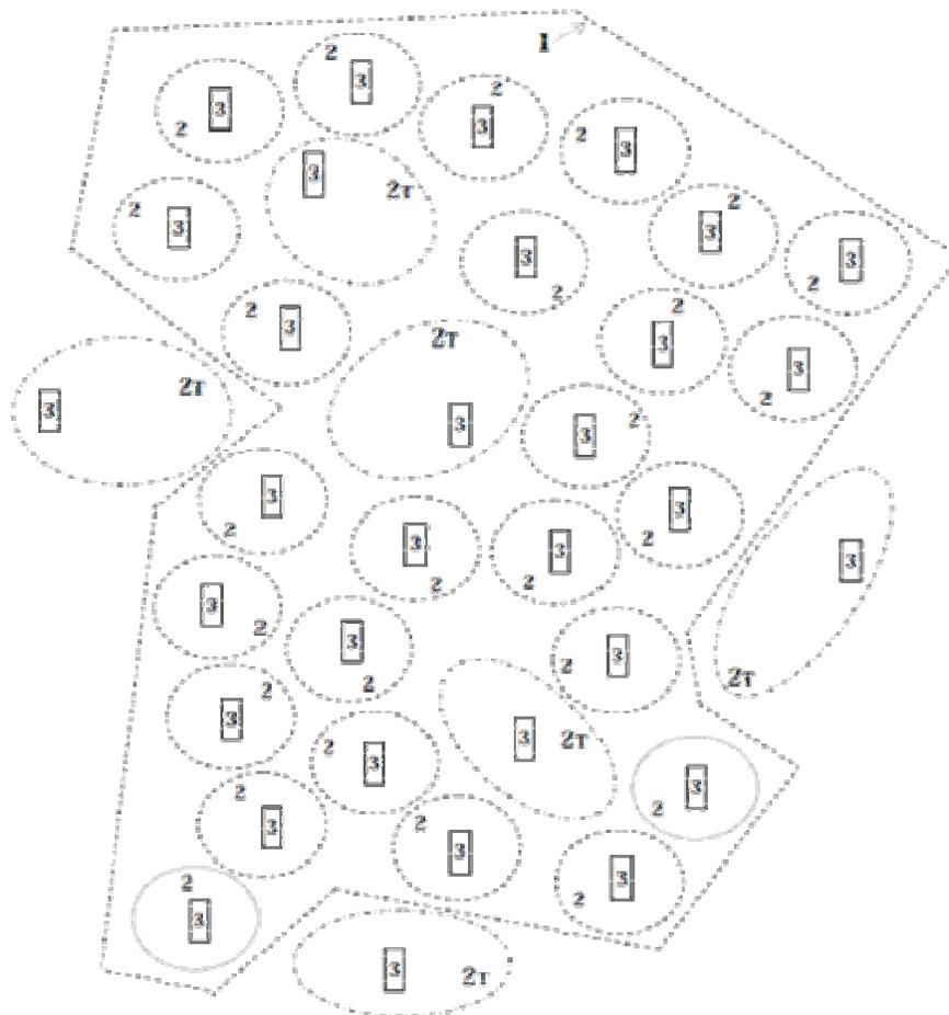
**Figure 2** An outline of a version of wide-ranging anti-hail protection network 1 – a protected area, 2 – a protected site, 2T – a trapping area, 3 – an anti-hail protection system
