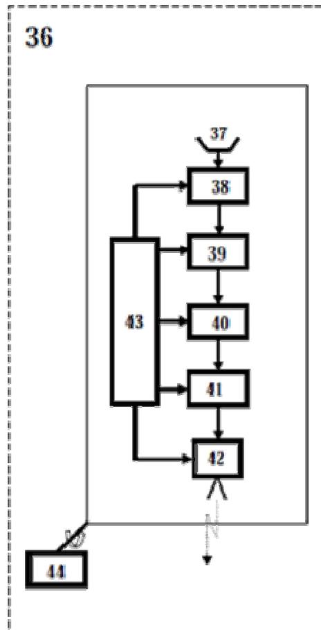
**Figure 6** A block diagram of a far-range detector-alerter 36 – a far-range detector-alerter, 37 – a far-range antenna, 38 – a far-range radiometric receiver, 39 – a far-range compensation device, 40 – a single-channel thresholder, 41 – a far-range warning device, 42 – a far-range transmitter, 43 – a far-range power supply, 44 – a scanner
