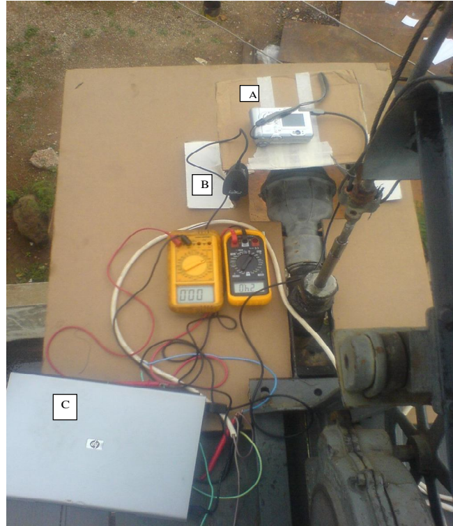
Figure 3. Photograph of the set up to measure voltage and current of motor and the flow rate simultaneously, showing: A-Camera recording flow meter, B- Camera recording Ammeter and Voltmeter and C- the computer.
