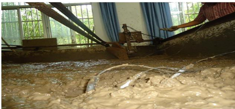
Figure 6 (a) Soil deformation sensor buried in soil
