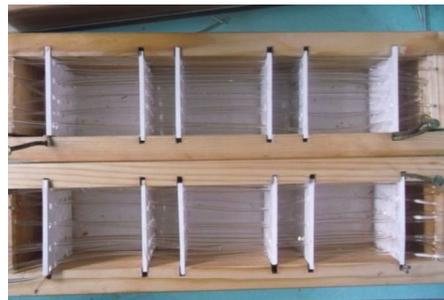
**Figure 1.2** wooden compressive moulds
