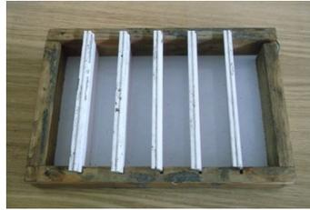
Figure 1.4 wooden flexure moulds
