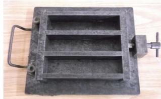
Figure 1.5 metal flexure moulds
