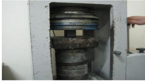
Figure 1.8: Cubes during compression test
