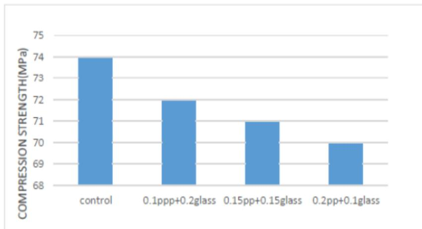
Figure(4c): compression strength containing combined polypropylene and glass fiber
