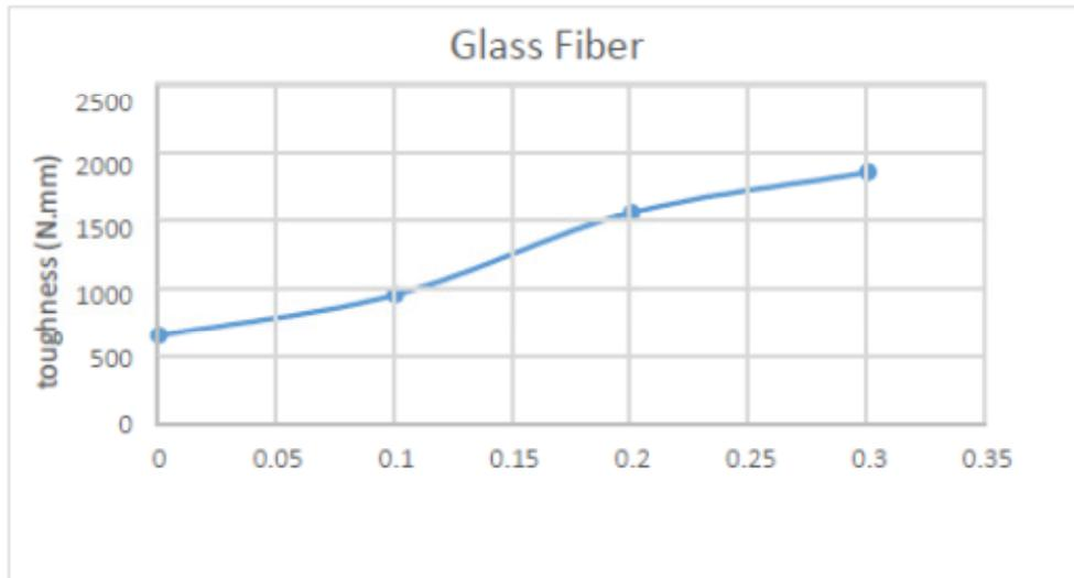
figure (8b) : toughness of specimen containing glass
