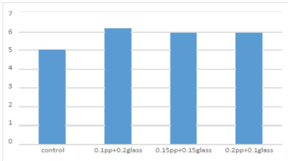
Figure(7c): bending strength combined polypropylene and glass fiber
