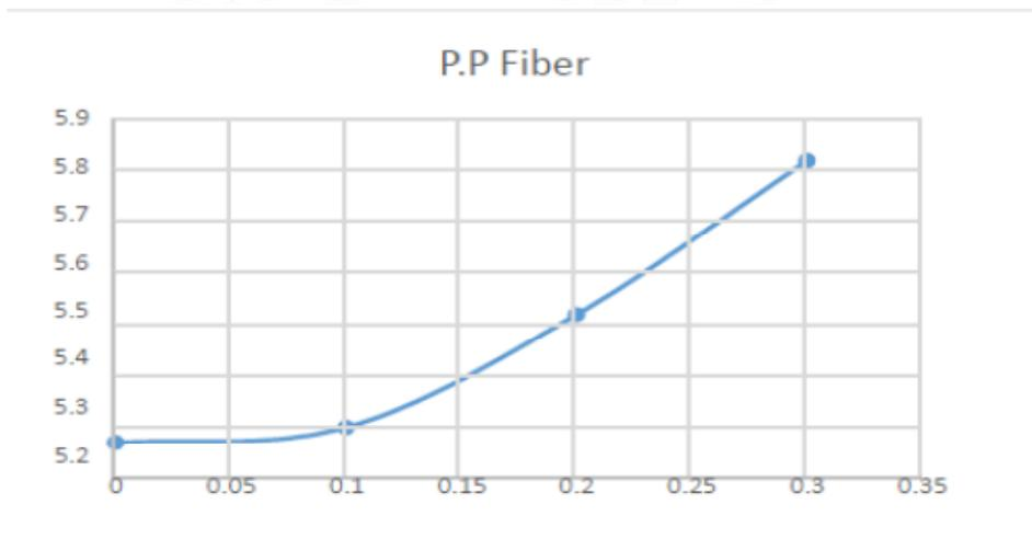
Figure (7a) : bending strength of specimen containing polypropelene
