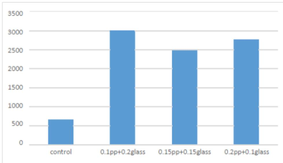
Figure(8c): toughness of combined polypropylene and glass fiber
