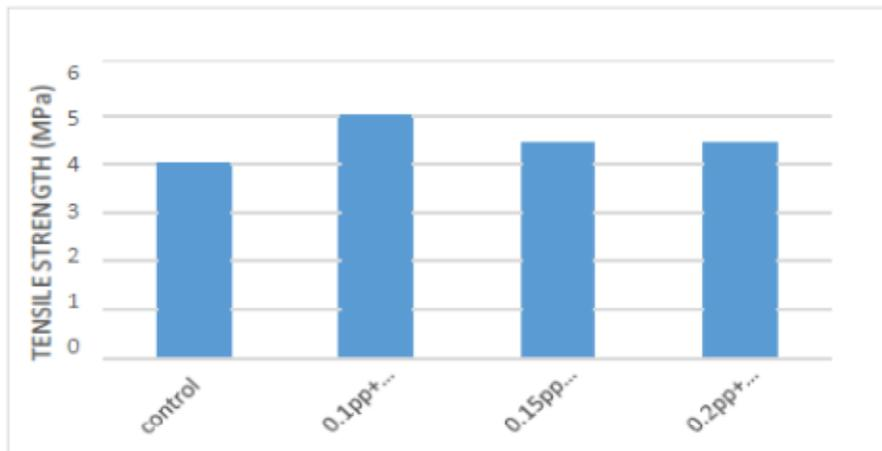
Figure(5c): tensile strength containing combined polypropylene and glass fiber
