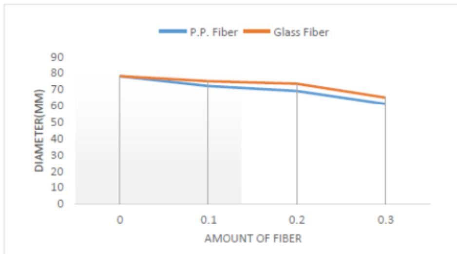
Figure 2. slump test on combined polypropylene and glass fiber
