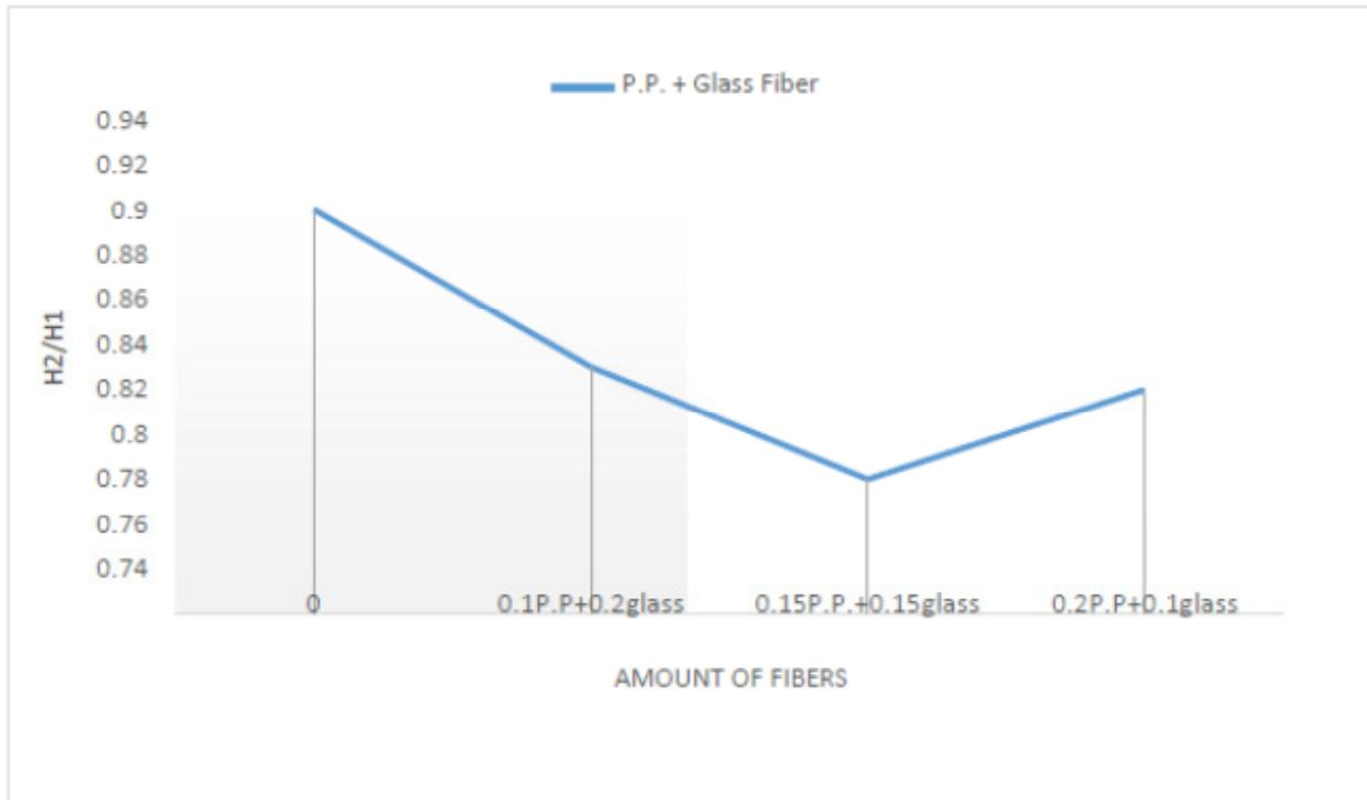
Figure (3b). L-BOX on combined polypropylene and glass fibers
