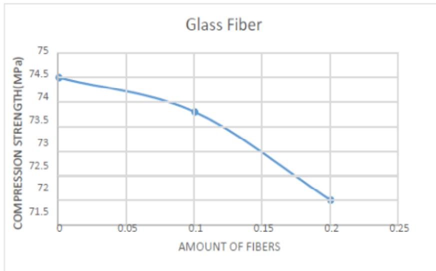
Figure (4b): compression strength of glass fiber
