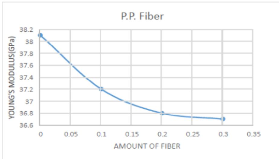
figure (6a) : young's modulus of specimen containing polypropylene
