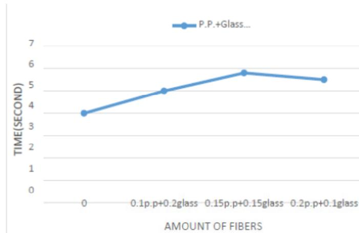
Figure (1b): slump flow test (T50) on combined polypropylene and glass fiber
