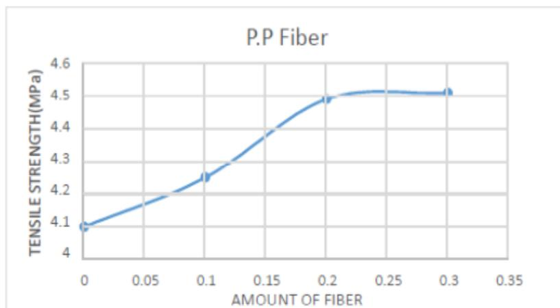
Figure(5a): tensile strength of polypropylene
