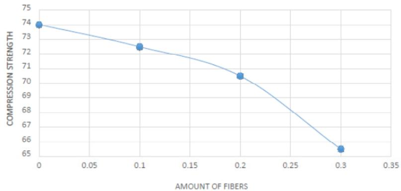
Figure(4a) : compression strength of polypropelene
