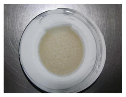
Figure 1. Aspect of the filter membrane after one water purified sample was filtered.
