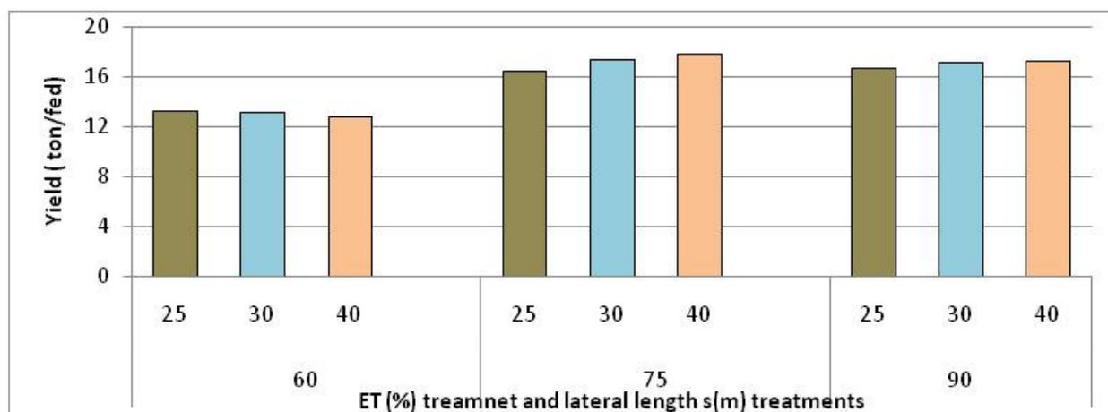
Figure 2: Onion yield as affected by irrigation treatments ET%) and lateral length (m)
