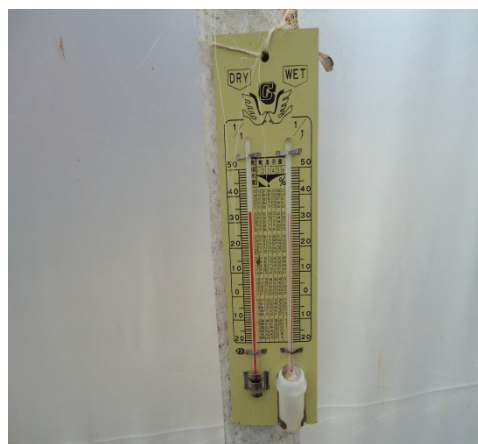
Figure 2. Wet and dry bulb thermometer
