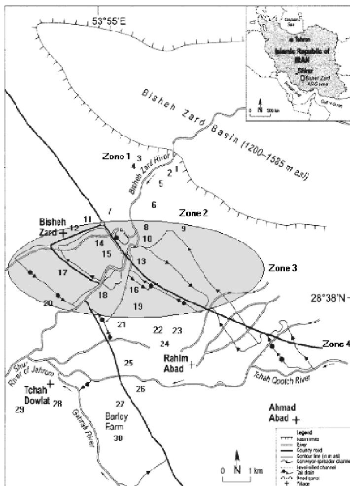
**Figure1.** Sketch map of the Gareh Bygone Plain (GBP) artificial recharge of groundwater (ARG) systems. Numbers denote production wells; the grey oval denotes ARG systems in the study area.
