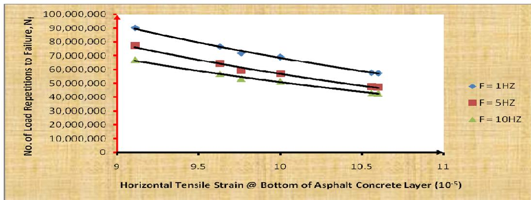
Figure 2. Variation of No. of Load Repetitions to Failure with Horizontal Tensile Strain
