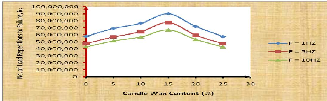
Figure 1. Variation of No. of Load Repetitions to Failure with Candle Wax Content
