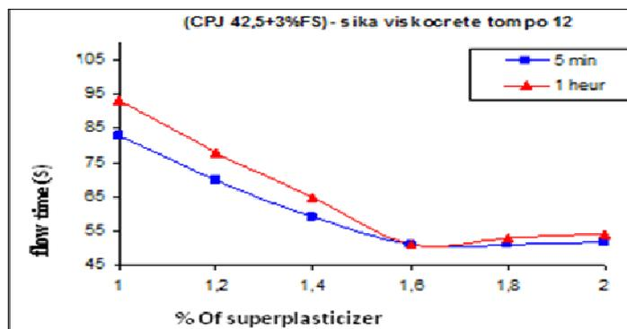
**Figure 1.** pair bonding (CPJ42.5 3% FS) - Sika Viscocrete tompo 12
