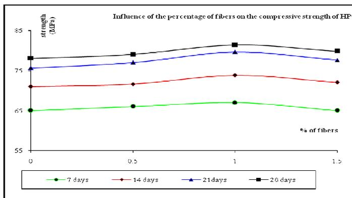
**Figure 2:** Effect of metal fibers % on the compressive strength of high-performance concrete
