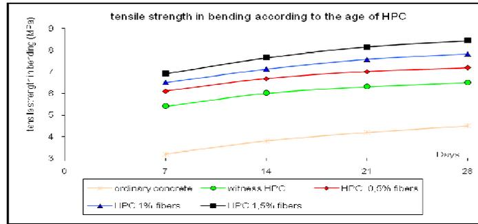
Figure 3. Results of the evolution of the tensile strength by bending of HPC versus time (days)
