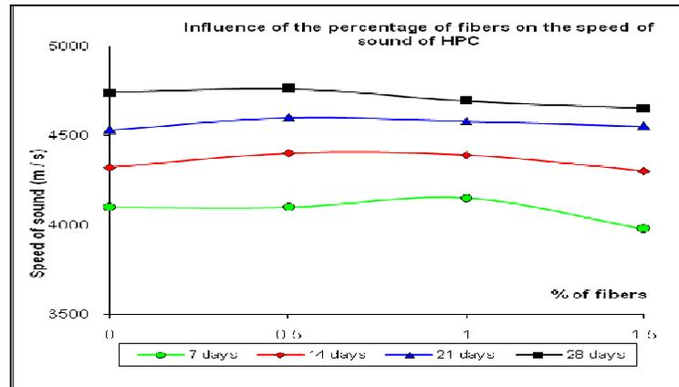
Figure 7. Effect of % of fibers on the speed of sound
