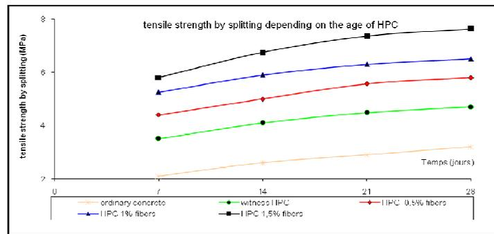
Figure 4. Results of the evolution of the tensile strength by splitting of HPC versus time (days)
