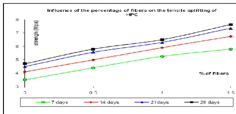
Figure 6: Effect of metal fibers on the splitting tensile strength at different ages of HPC
