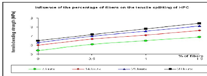
Figure 5: Effect of metal fibers % on the flexural tensile strength at different ages of HPC
