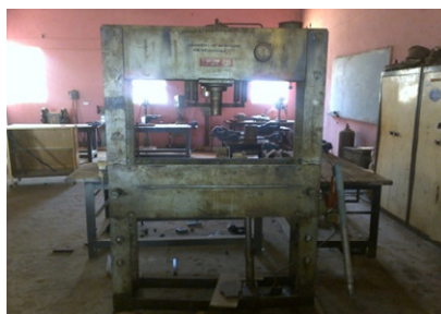
Plate 2. Hydraulic Press used for the oil Expression
