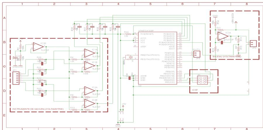
Figure 2 Voltammetric Amplification Module (M1), Scan mode, Analog-to-digital serial interface Module (M3)
