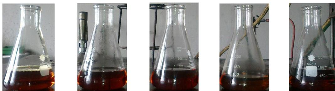
**Figure 3.** Color of different bio-diesel blends (without Transesterification), and pure mustard oil.
