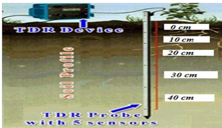
Figure 3: TDR device and probe with five sensors
