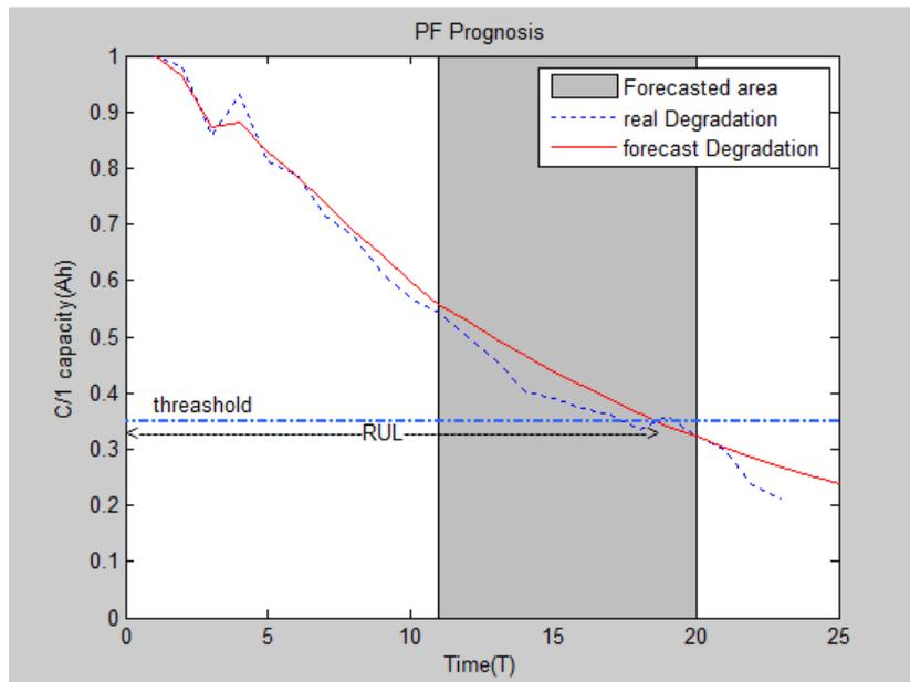
Figure 4. Trajectory of degradation for the cell of battery pack using Particle Filter
