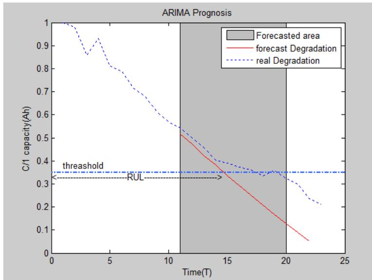
**Figure 5.** Trajectory of degradation for the cell of battery pack using ARIMA model
