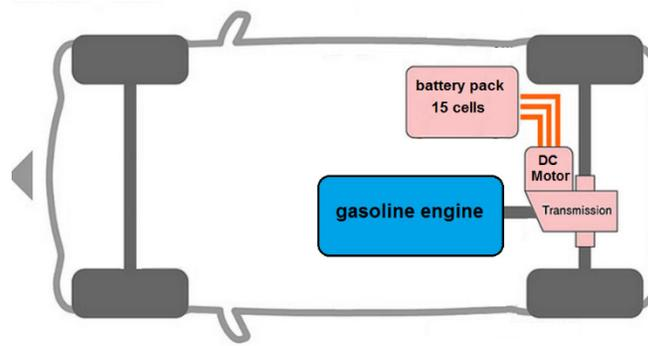
Figure 3. Plan of Hybrid Electric vehicle
