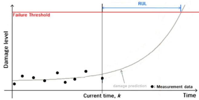
Figure 1. illustration of RUL calculation
