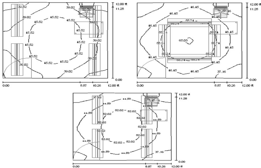
Fig1.3 Illuminance diagrams of Luminaire Arrangements 1, 2 and 3
