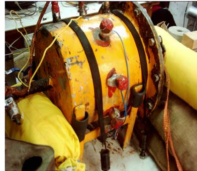
Figure 3. the outer structure of combustion chamber
