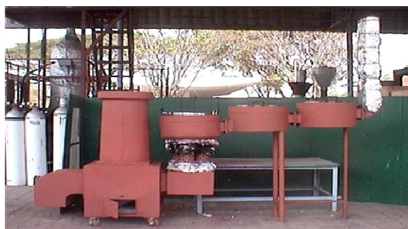
Fully assembled Gasifier Stove CGS3 with pot support
