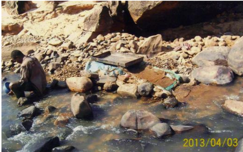
Figure 5. Traditional Sand Washing Method
