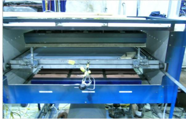
Figure 8. Experimental set-up of a Thermoforming oven
